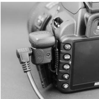
An optional remote control accessories (2.5mm jack) can be connected to the remote terminal of ECO PS-2 GPS for remote shutter release.
