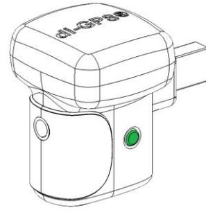
The **GPS** icon will stop blinking once signal has been established and the camera is ready to record the current position.
